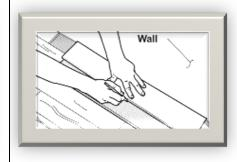
The last row (possibly the first row) plank width should be no less than 50mm (2") on the long seam.
