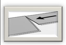
Install the second piece in the first row by laying the short end tongue onto the previously installed piece short-end groove.
